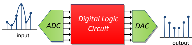
Figure 4.3: Block diagram of a general system developed in this chapter.
